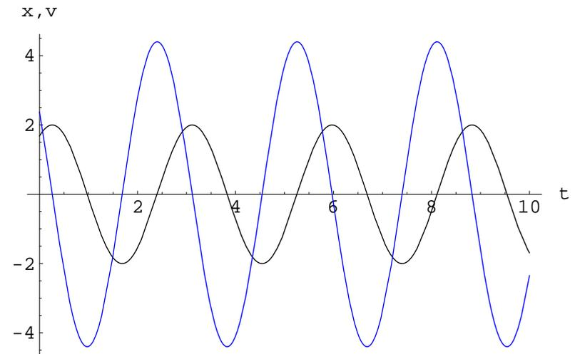
振幅  $A = \sqrt{C_1^2 + C_2^2}$  [m]
